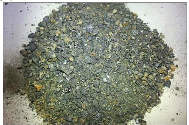
Above, galena with associated gangue & right, the same sample after crushing.
