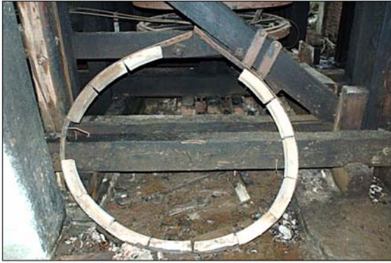
The pulley had a wooden friction brake. The picture shows a brake detached from the pulley.
